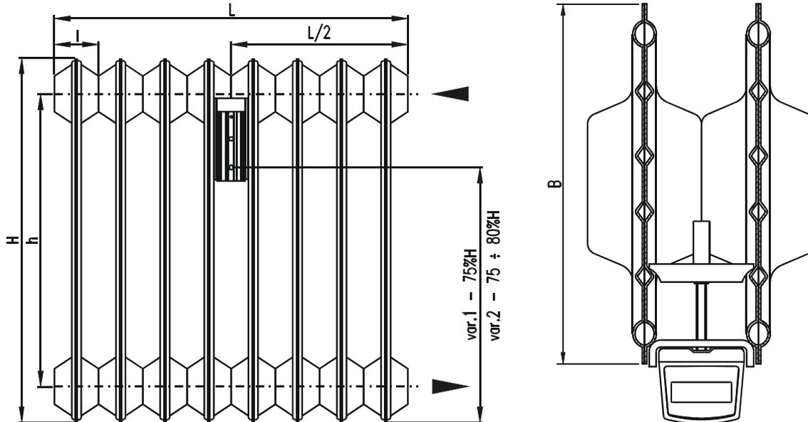
Basic dimensions of the SVRATOUCH 500/160 for 10 segments, data for correct allocator installation (mm):
