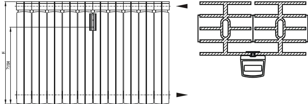
Basic dimensions of the SOLAR 500 radiator and data for correct allocator installation (mm):
