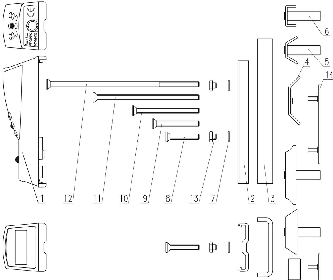
Illustration 8: E-ITN 30 Mounting material for segmented radiators
