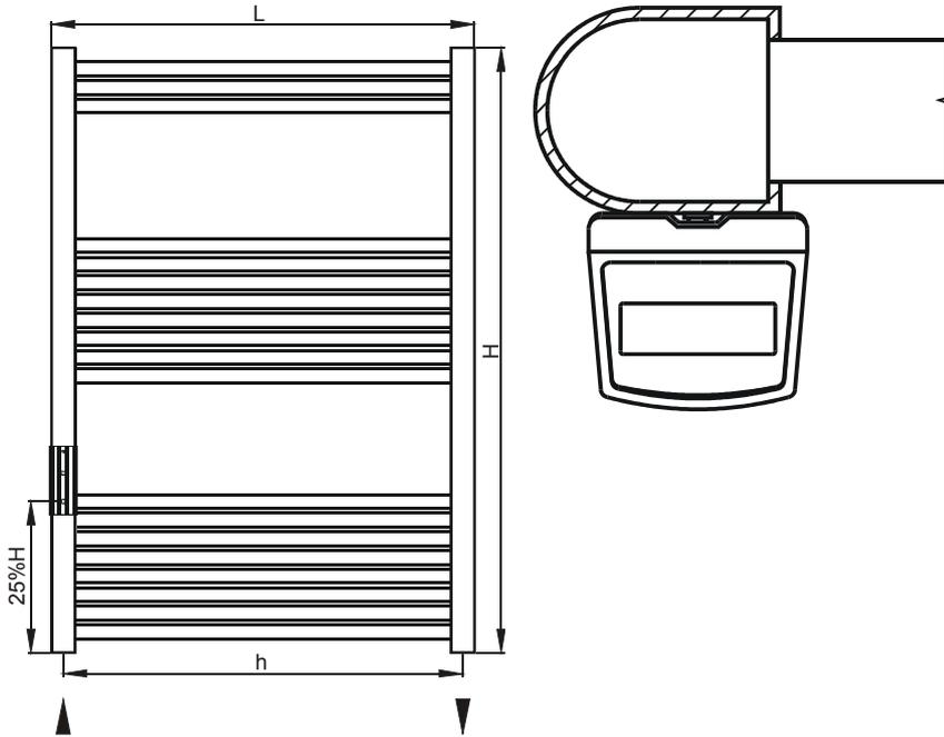
Basic dimensions of the K 750/1640 radiator and data for correct allocator installation (mm):
