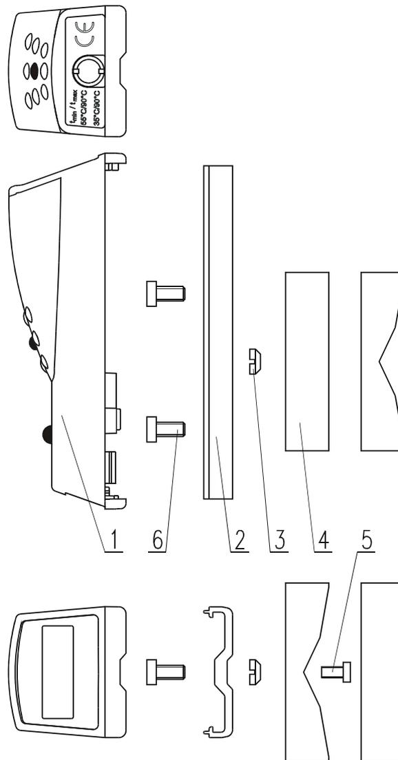
Illustration 10: E-ITN 30 Mounting material for tubular radiators
