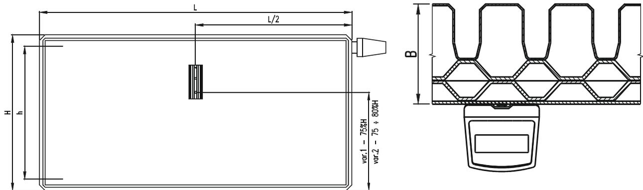
Basic dimensions of the RADIK, VENTIL KOMPAKT modification, type 11 PLAN VK and data for correct allocator installation (mm):
