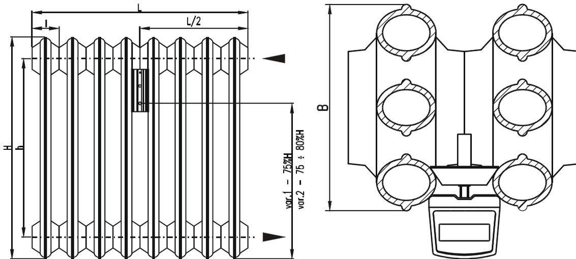
Basic dimensions of the KALOR – 500x110 for 10 segments, data for correct allocator installation (mm):
