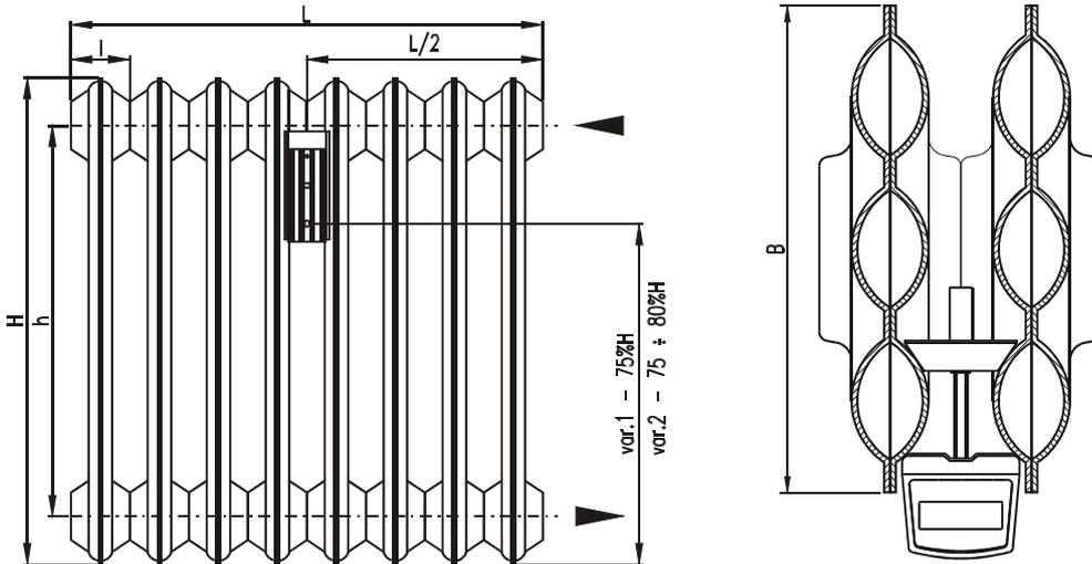
Basic dimensions of the NERIA 500/150 for 10 segments, data for correct allocator installation (mm):
