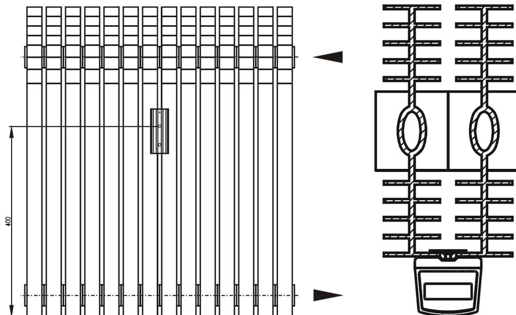
Basic dimensions of the FONAL A 650-175 and data for correct allocator installation (mm):
