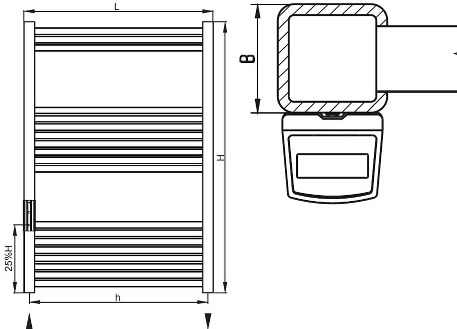
Basic dimensions of the K 750/1640 and data for correct allocator installation (mm):
