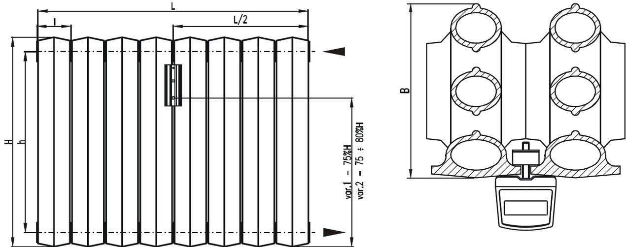
Basic dimensions of the KALOR 3 for 10 segments, data for correct allocator installation (mm):
