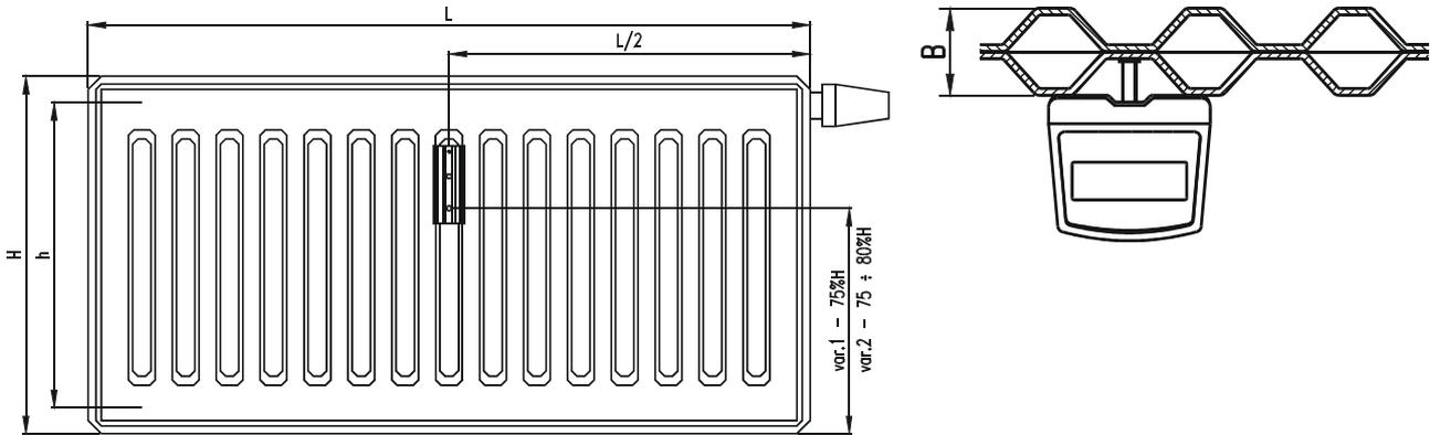
Basic dimensions of the RADIK, KLASIK modification, type 10 and data for correct allocator installation (mm):
