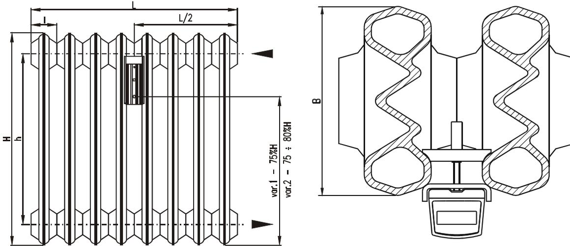
Basic dimensions of the S-130 for 10 segments, data for correct allocator installation (mm):
