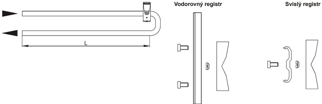
Steel registers are used only in areas with low hygiene and esthetic requirements. Dimensions are chosen accordingly to needs. Registers are usually made accordingly to drawings attached with project. Mounting material can be used for pipes from  $\varnothing$  30 to  $\varnothing$  110 mm.
